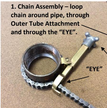
1. Chain Assembly – loop chain around pipe, through Outer Tube Attachment and through the “EYE”.
